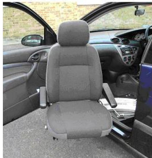
Seat that rotates at an angle of 180 degrees outside and alongside the vehicle.
