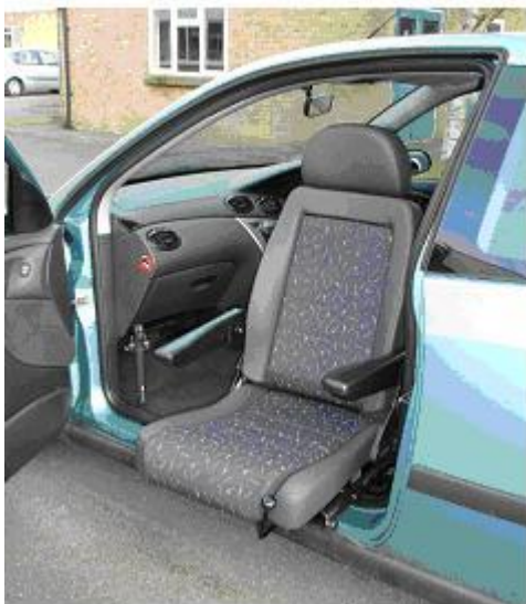
Seat that rotates at an angle of 90 degrees outside the vehicle.
